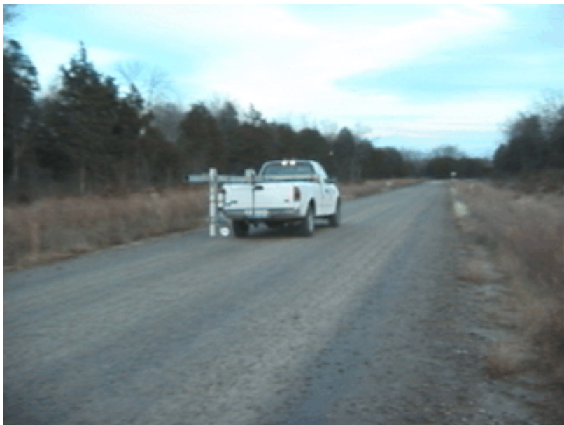
Figure 6. Truck with Mobile Sampler on Treated Road
